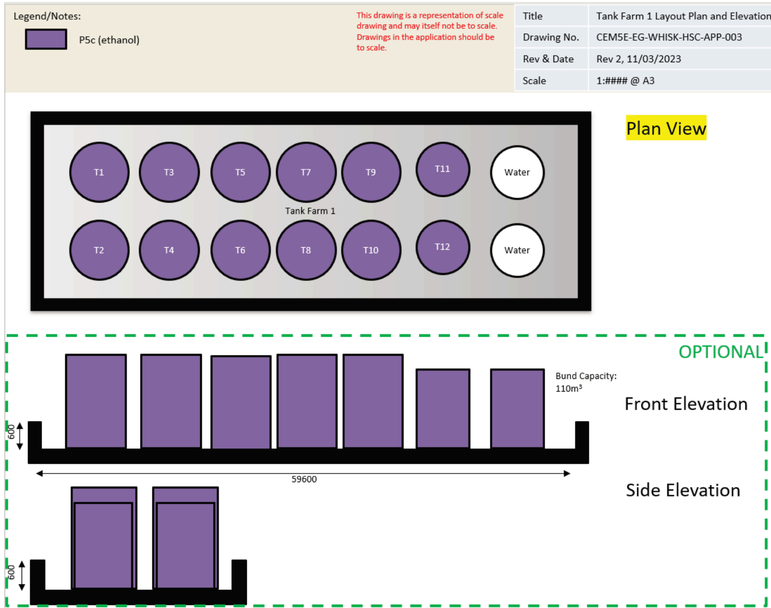
Figure 4 Substance Location Plan for Tank Farm
